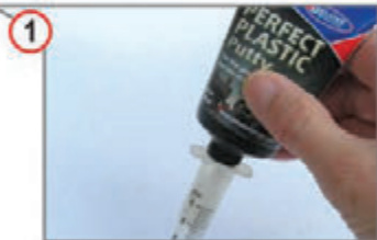
1 Fill a Pin Point syringe from Deluxe Materials; this allows fine application of the putty.
