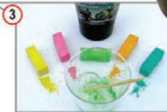
3 Adding colour to Perfect Plastic Putty is easy by adding pastel chalk scrapings until you get your colour.
